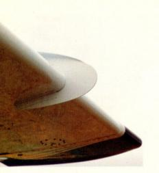
Vortex generators mounted on the wing leading edges further remind you this is no run-of-the-mill 206.
