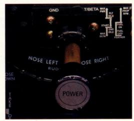
Soloy says it takes a few hours to become accustomed to the operation of the power lever (above). The schematic shown on the placard to the right of the power lever shows the basic motions needed to position it for start, ground idle, beta, flight idle, and maximum power.
