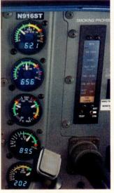
The airplane flown for this report was fitted out with Garmin's G500 retrofit primary flight display and multifunction display and dual Garmin 530s. Vertically stacked engine gauges (above) keep track of engine parameters such as the all-important turbine outlet temeprature. The rectangular, vertically oriented annunciator panel to the right of the engine gauges is another part of the Soloy mod. Among other items, it indicates when the propeller is in beta or reverse pitch.
